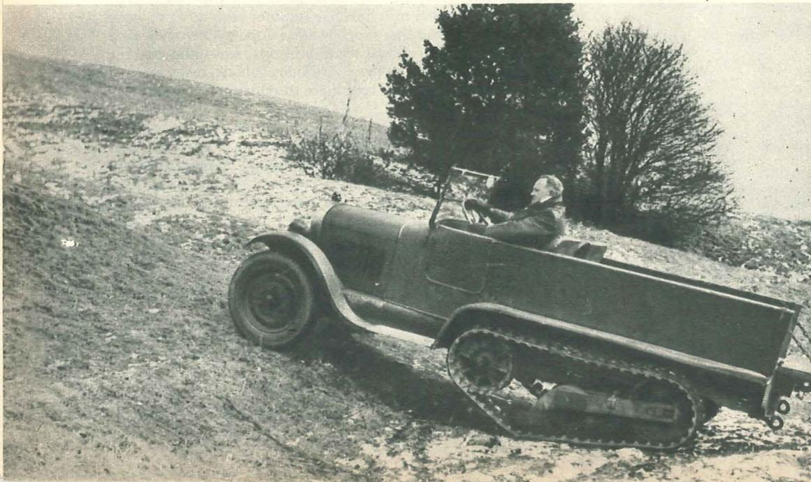
Good ground clearance, little rear overhang, and flexibly-swinging rear tracks enable the car to tackle really rough country without grounding. Its rubber tracks also make it quite at home on normal roads.
