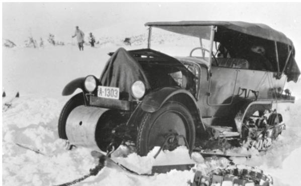
4 pictures from Hedemark Museum. All are taken in 1935 during a trip in the mountains. The P17 car broken down, the rubber track probably not resist. P17 was towed by a P15N and mounted on a transport truck.
