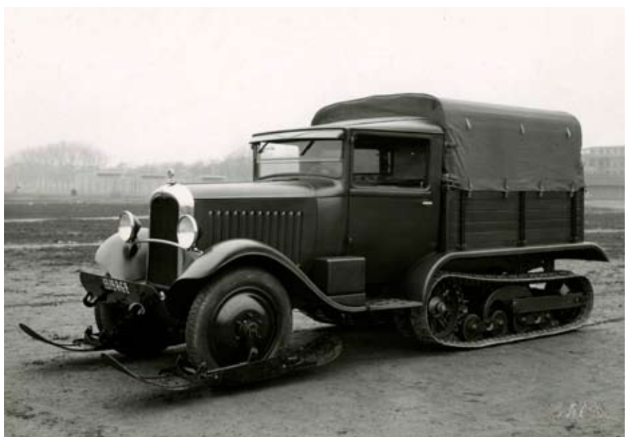
The front pulley has a larger diameter than the rear one on the P15 NK.
