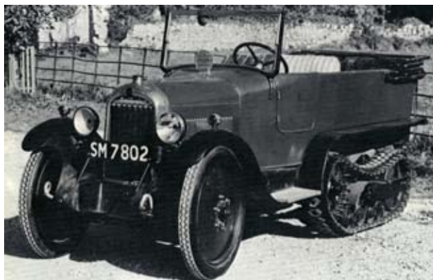
Early P10 (or late P7bis?). This car is in the British National Car Museum. The radiator looks like the B14, but with its 8 separate elements, it is a special design for the half-track car.
