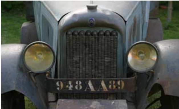
Radiator design of later P17 with 8 separate elements.
