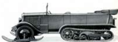
The front pulley has a larger diameter than the rear one on the P15 NK.
