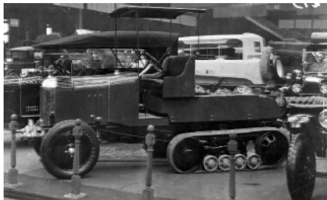
With the Citracit car in the background: Another P6, but with the tracks of type P4T. Similar cars are seen as fire engines and army vehicles.
