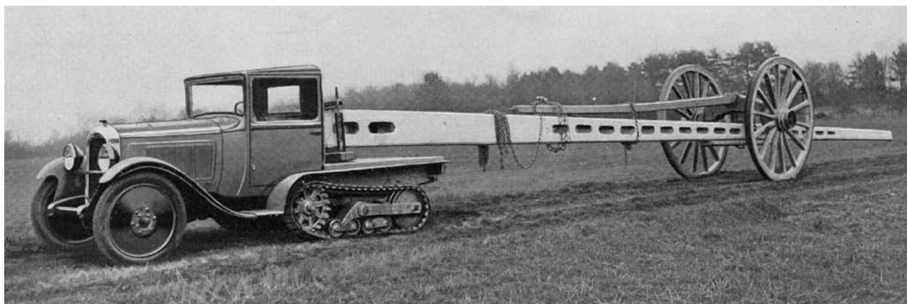
Early P10 (or late P7bis?). This car is in the British National Car Museum. The radiator looks like the B14, but with its 8 separate elements, it is a special design for the half-track car.
