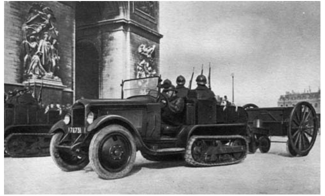
One of several hundreds French army cars. The wheel system for the cannon is another Kegresse patent.
