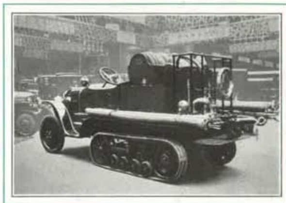
Citroën-Kégresse car fitted with high-power fire extinguishing appliances.
